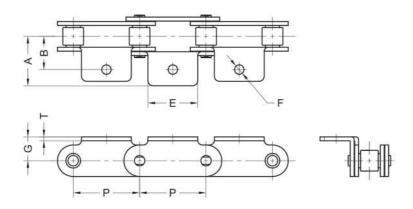
K-1 Bent two sides with one hole in each tab
