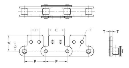
SK-2 Straight two sides with two holes in each tab
