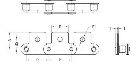
SK-1 Straight two sides with one hole in each tab
